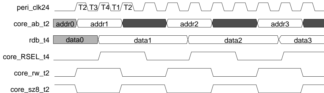
Figure 7-7 Basic 16-bit Core Register Read Timing
