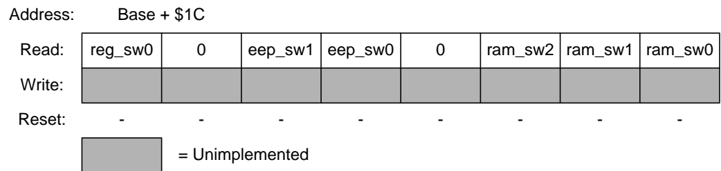
Figure 11-9 Memory Size Register Zero
