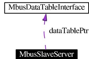
The base class **MbusSlaveServer** contains a protocol unspecific Server Engine and the protocol state machine. All protocol flavours inherit from this base class.
