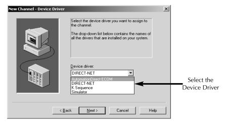
If the selection is the **AutomationDirect ECOM** driver., the wizard will prompt you to select a "Network Adapter". Click on the arrow to open the drop down list. This list shows the network adapters which are installed in your PC. Either select the adapter you wish to use or select **Default** and allow the operating system to select the adapter.
