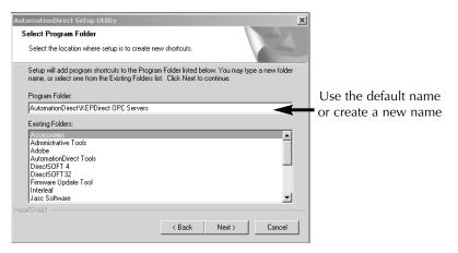
The window shown below appears. Verify the folder name where the KEP*Direct* files are to be stored. If this is the selected folder, click on the **Next** button to continue with the installation.
