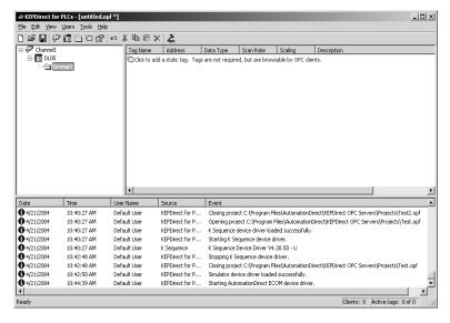
Tag groups can be added at any level from the device level down. Multiple tag groups can be nested together to fit the needs of your application.
