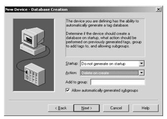
The **Startup** selection allows you to configure when OPC tags will be automatically generated. There are three possible selections:
