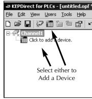
Once the channel setup is complete, the application window displays a directory tree on the screen showing the newly created channel name. Directly beneath the channel name is a device symbol. Either click on the text next to the symbol, **Click to add device**, or click on the **Add Device** tool on the tool bar to initiate the add device setup.
