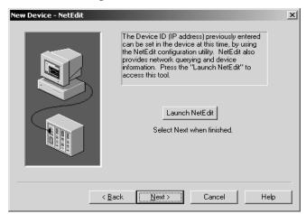
previously entered for the device, can now be set in the device. If you have previously set the ID in the device, this step can be bypassed. Clicking on **Launch NetEdit** will open the NetEdit window below.
