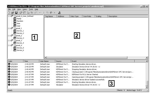
When the KEP*Direct* for PLCs Server application is launched for the first time, it opens with an operational simulation program. This is a sample program which can be used to practice adding devices and channels. The window is divided into three areas as explained below (see the window above for reference):
