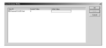
The cursor will be blinking in the **Write Value** area of the window. Type the number "1" and click on the **Apply** button. The Write Value now displays a "1" reflecting the "Synchronous Write" that was just applied and the **Current Value** displays a "1". The indicator for the output point just written to should now be illuminated on the PLC. Follow the same procedure to write a zero to turn off the output.
