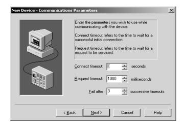
This screen provides three different communication settings for the device being installed. The following list explains the purpose of each available setting.
