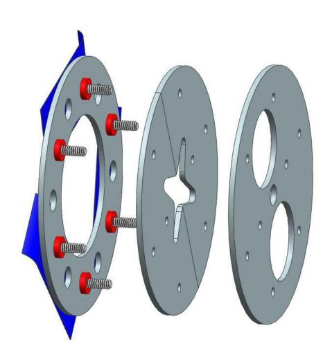
BE SURE that the two small holes in the center line up!
