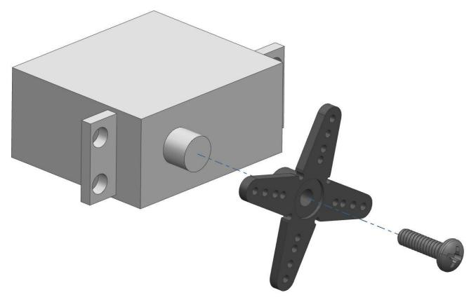
Put the screw back into the servo when the horn is off.
